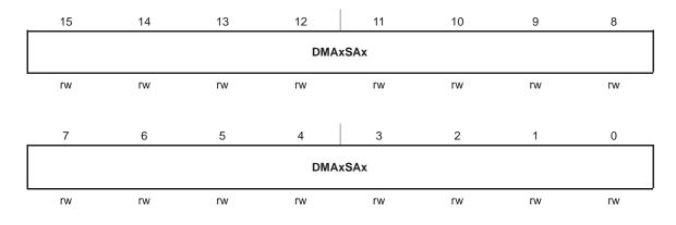
DMAxSAx Bits DMA source address. The source address register points to the DMA source address for single transfers or the first source address for block transfers. The source address register remains unchanged during block and burst-block transfers.
